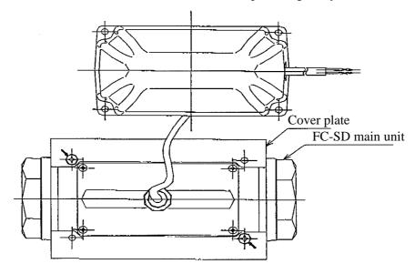
4. Slide and remove the cover plate from the main unit.
