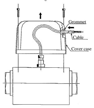
3. Remove the two screws that secure the cover plate diagonally.
