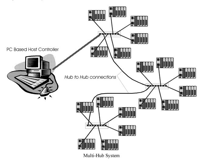
In a multi-hub system, all connections between the PC and a hub, or an RTU and a hub are straight-through. All connections between hubs are crossover.
