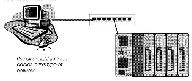
In either configuration, the first thing to check is if "Link" lights appear on the RTU. If you are connecting through a hub, link lights should appear on both the RTU connection and the PC connection. If the link lights do not appear you probably have a bad connection.
