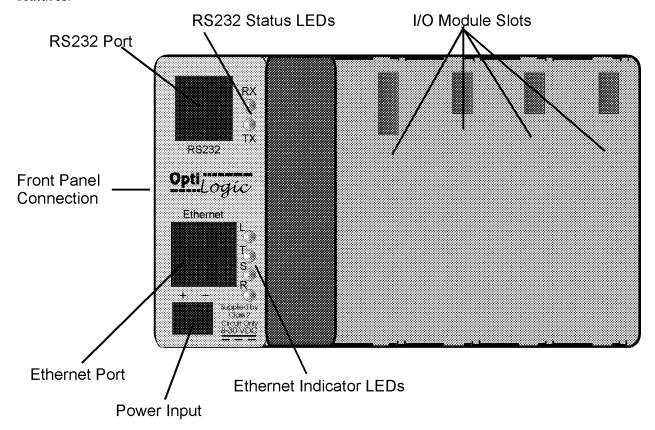
receive (RX) are active. The Ethernet port provides indications for good Ethernet link standard DIN rail. It also can snap onto the DIN connection (L) and Ethernet port access by the base processor (S) as well as transmit (T) and receive (R) indicators.
