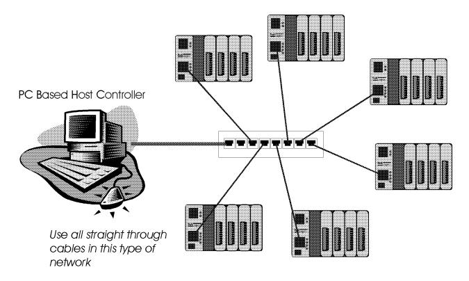
Crossovers are made internal to the hub. Therefore, in a single hub system, all connections are straight-through. Remember that for 10Base-T, each cable connection is limited to 100 meters in length.
