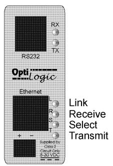
The first thing that happens when the RTU is powered up is that is checks its operating This process takes a couple of program. If the operating program does not check out, the RS232 TX (transmit) LED will flash at a rate of about 1 flash per second. If this should happen, the base must be loaded with operating software.
