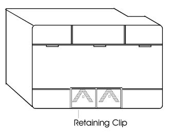
As shown in the figure, there is a DIN rail channel that runs lengthwise across the middle of the RTU base's bottom side. At the top of that channel are three overhanging hooks. At the bottom of the channel there is a sliding retaining clip.
