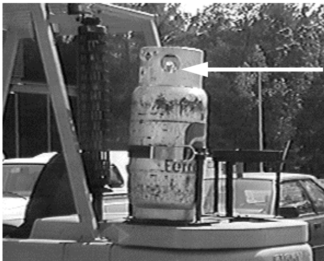
This is a propane tank, found on a propane powered forklift. The valve is located on top of the tank.
