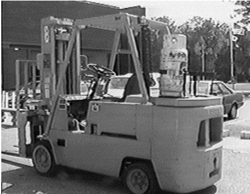
Example of a propane powered forklift found at Jefferson Lab.
