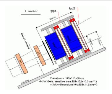
Double analyser FPP used to extract beam-helicity asymmetries at spectrometer focal plane.
