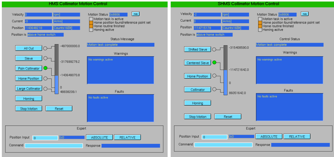
Figure 4.9: HMS and SHMS slit system screens in normal operation.
