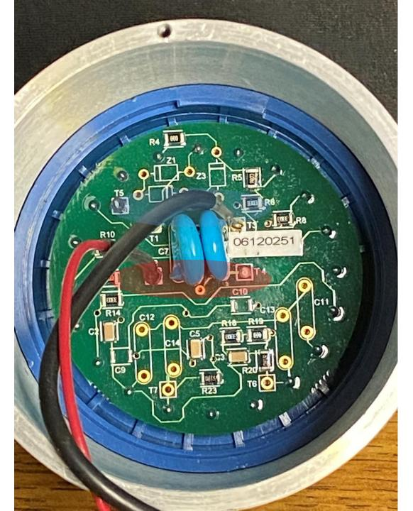
Because the board is recessed in its big blue socket, the near-spikes on the periphery are ~8mm from the grounded metal casing. <u>And they</u> were coated after the board was stuffed.\* So I'm not too worried about these near-spikes.
