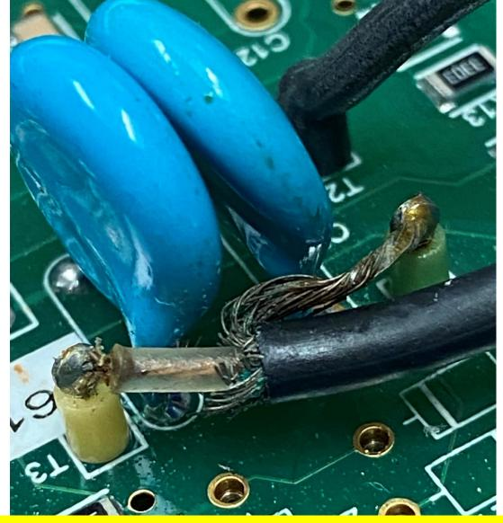
In a brief test at 2300V in air, I could not make this base spark. That's expected, since an air gap would have to drop to only ~2mm to start sparking infrequently.
