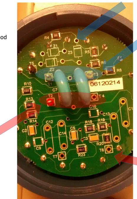
I've marked low potential areas with **blue**, and high potential with **red**. Potential increases systematically with resistor number.
