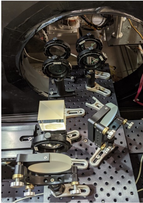
(c) Longitudinal optics alignment on the top table.
