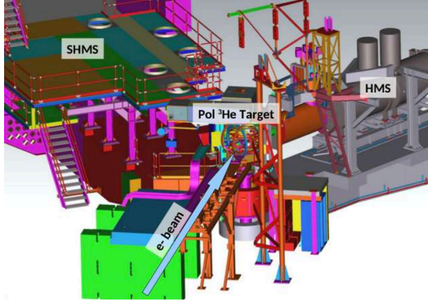
Figure 3.1: Setup for experiment E12-06-110 in Hall C.
