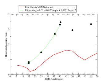
Figure 1: HMS horizontal pointing versus HMS angle. The fit is to the data points at 40 degrees and below. Eric Christy's HMS data set is from the 6 GeV measurements.
