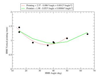
Figure 2: HMS vertical pointing versus HMS angle. The red line is fit to data up to 50 degrees and is used in HCANA. The green line is fit to all the data points.
