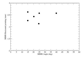
Figure 3: SHMS horizontal pointing versus SHMS angle.
