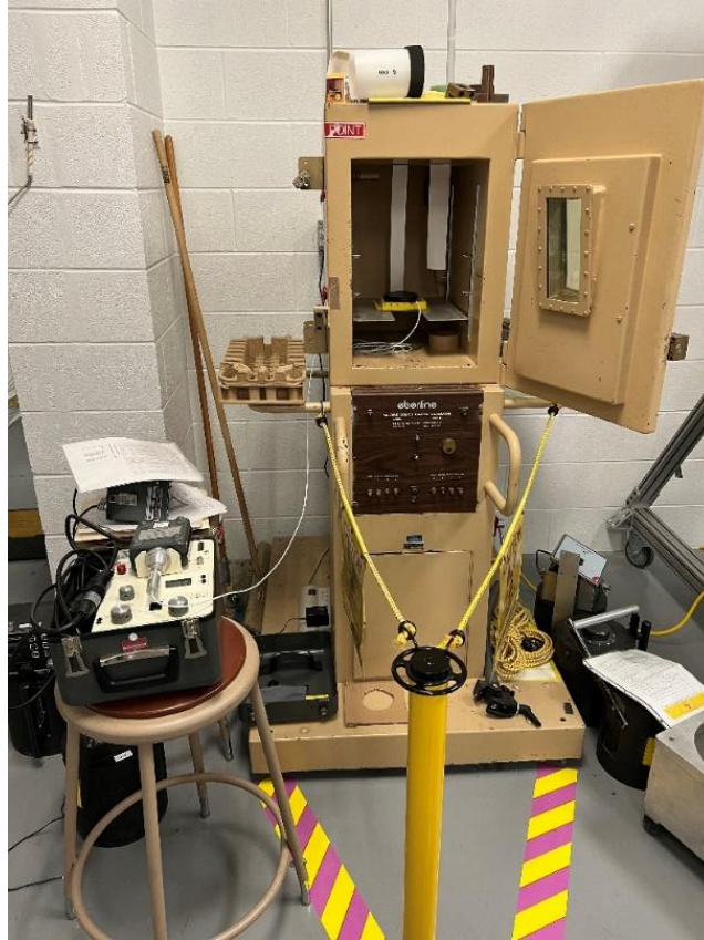
Figure 2 Cs-137 irradiator cabinet (before we moved in). When the door is shut and locked, and the shutter control rods are unlocked and pulled, a somewhat conical beam of beta and gamma rays comes out of a hole in the floor of the cabinet.
