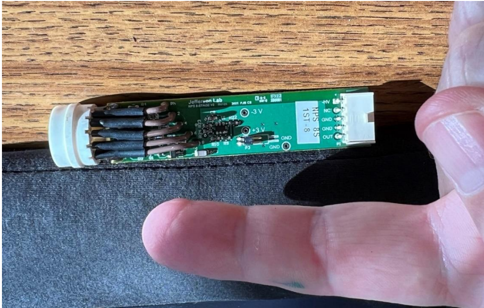
Figure 1 Amplifier side of a base. The two +3V test points are clearly visible, along with a convenient ground. The two voltage regulation chips are on the other side of the board.
