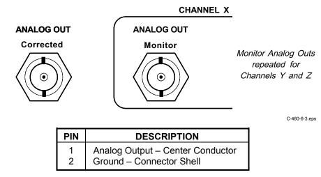
Figure 6-3. ANALOG OUT Corrected and Monitor BNC Connector Details
