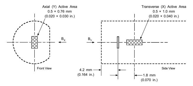
**NOTE:** Active area is defined as the portion of the Hall plate where the majority of magnetic sensitivity occurs. All position dimensions of the active area adhere to a tolerance of  $\pm 0.25$  mm (0.010 in.). Each active area is perpendicular to the other two to within  $\pm 0.5^{\circ}$ .
