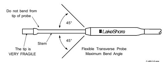
Figure 3-5. Maximum Flexible Probe Bend Radius
