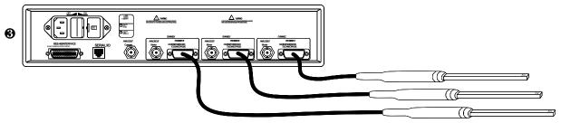
The Model 460 configured as 3 separate gaussmeters.
