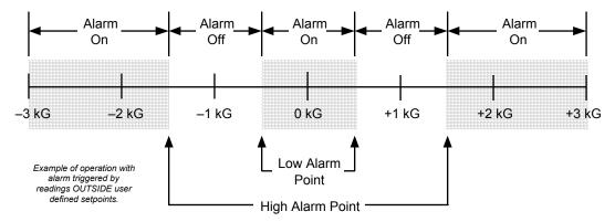
To enter this alarm setup, push the **Alarm Set** key. The user is first asked to enter the High Alarm Point as follows:
