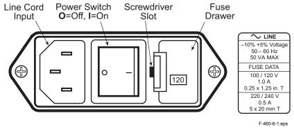
Figure 6-1. Power Fuse Access
