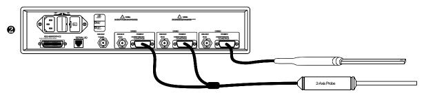
The Model 460 configured as 2 separate gaussmeters.
