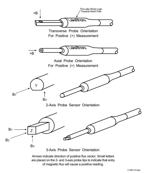
Figure 3-6. Probe Orientation For Positive Measurement
