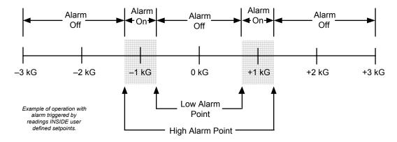
To enter this alarm setup, push the Alarm Set key. The user is asked to enter the High Alarm Point:
