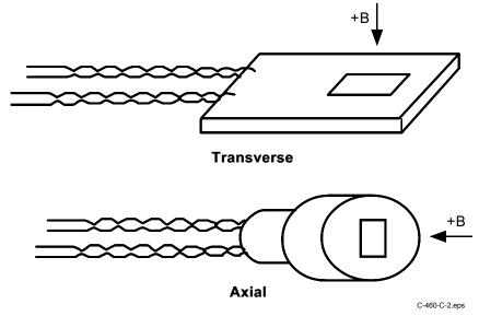
Figure C-2. Axial and Transverse Configurations
