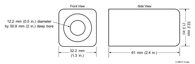
Figure 5-12. Model 4060 Zero Gauss Chamber
