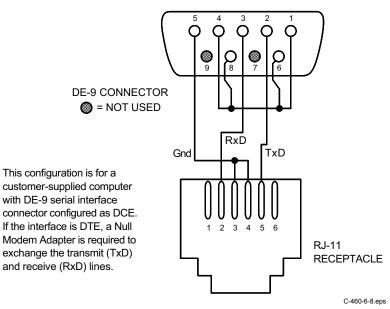
Figure 6-8. Model 4003 RJ-11 to DE-9 Adapter Wiring Details
