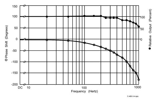
Figure 3-4. Monitor Analog Output Frequency Response
