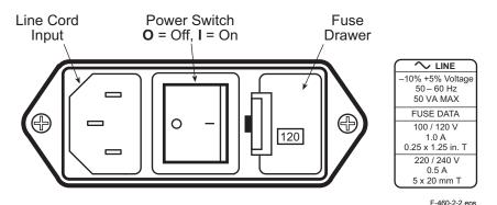
Figure 2-2. Line Input Assembly
