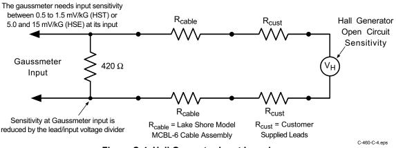
Figure C-4. Hall Generator Input Impedance
