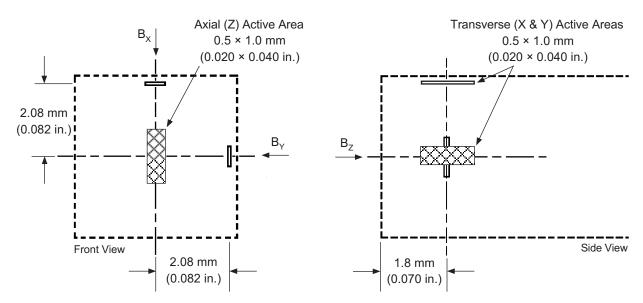
**NOTE:** Active area is defined as the portion of the Hall plate where the majority of magnetic sensitivity occurs. All position dimensions of the active area adhere to a tolerance of  $\pm 0.25$  mm (0.010 in.). Each active area is perpendicular to the other two to within  $\pm 0.5^{\circ}$ .
