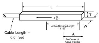
Small variations in, or low values of large volume magnetic fields, such as that of the Earth or fringe fields, around large solenoids, can be measured with these ultra-high sensitivity probes. Resolutions of several gammas (10<sup>-5</sup> gauss) to tens of gammas are available depending on the mating gaussmeter.
