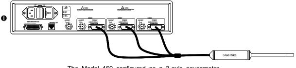
The Model 460 configured as a 3-axis gaussmeter.
