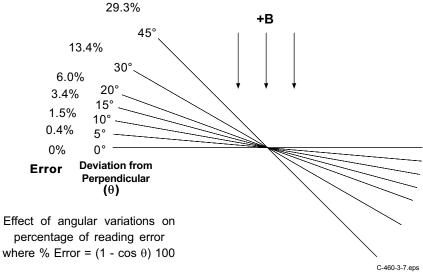
Figure 3-7. Effect Of Angle On Measurements
