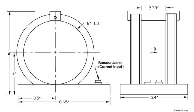
Figure 5-9. Model MH-6 Helmholtz Coil
