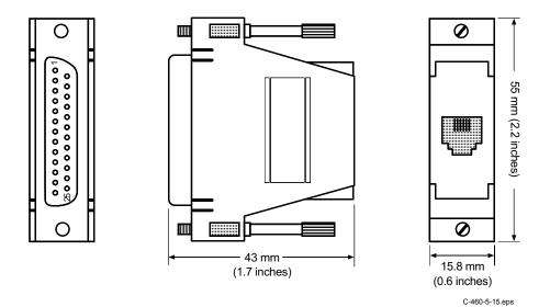
Figure 5-15. Model 4002 RJ-11 to DB-25 Adapter
