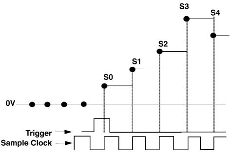
Trigger: Starts burst waveform generation
