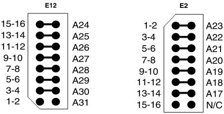
**Example 2:** This Jumper Configuration Gives a Base Address of 0x80000000 when E26 and E27 are properly configured.
