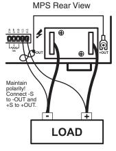
Figure 2-3. Remote Sensing Connections
