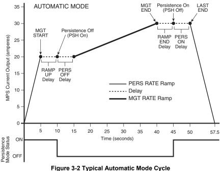
To pause a ramp or skip a time out, press either the Data Entry up or down key. To abort the operation, press **Escape**. After an abort, **<RUN>** continues an automatic process from where it left off.
