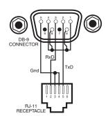
Figure 5-6. Model 2003 RJ-11 to DB-9 Adapter Wiring
