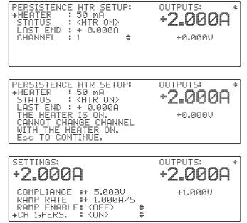
3. The selected current multiplied by the heater resistance ( $e = i \times r$ ) must be less than 15 Vdc for the MPS to accurately determine compliance of the switch heater (open resistance).
