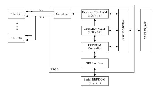
Figure 4: F1 TDC Configuration Control Logic
