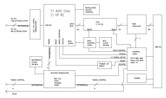
Figure 1 – F1TDC Module Block Diagram
