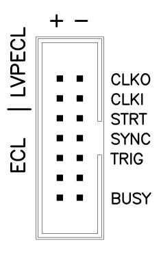
Figure 6 – Timing & Control Signals
