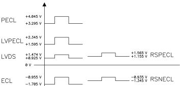
Figure 9 – Typical High-Speed Differential Signal Standards
