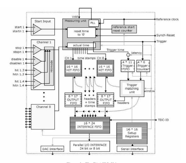
Figure 2 - The F1 ASIC Chip
