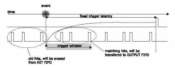
Figure 3 - Trigger Matching
