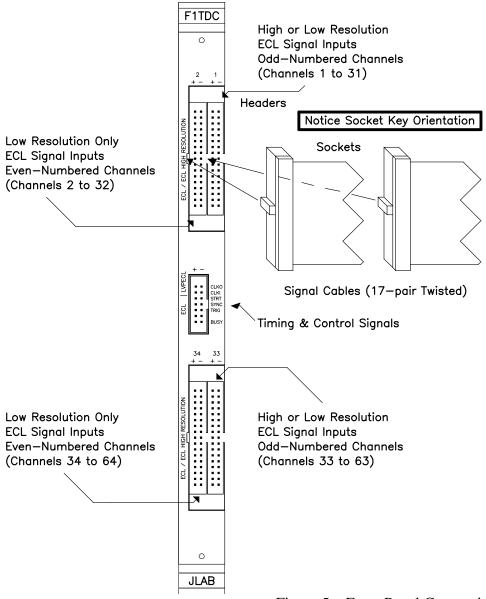
Figure 5 – Front Panel Connections
