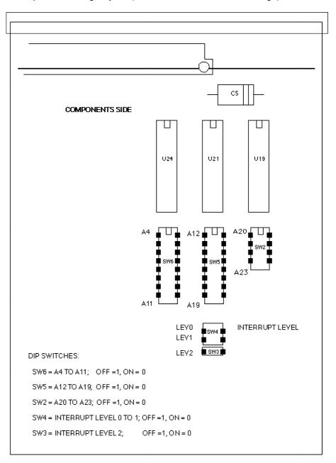
Fig 6.1 V288 dip switches setting
