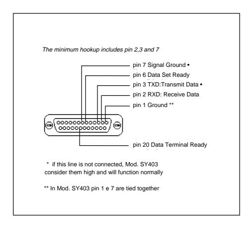
Fig 3.2 RS232 connector pin assignment
