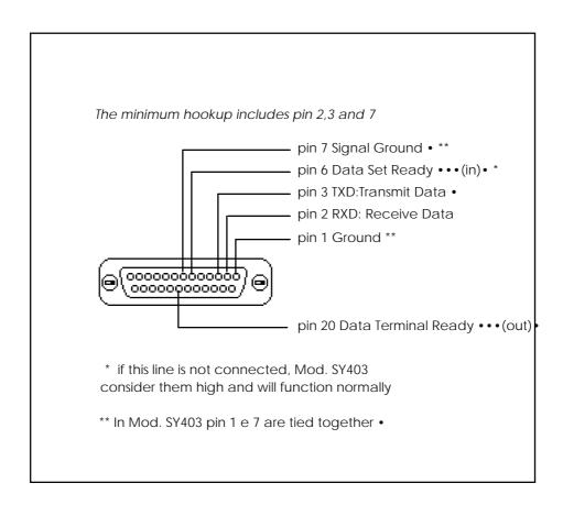
Fig C.1 RS232 connector pin assignment
