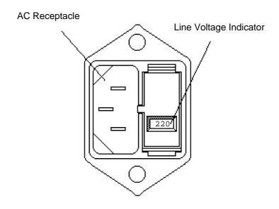
Fig C.2: Operating Voltage Indicator
