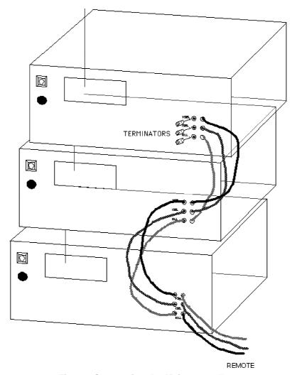
Fig. 3.1 Connecting the Main controllers
