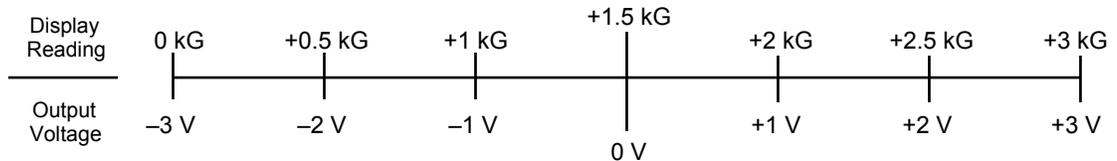
To enter this scale, press the **Analog Out** Key. Press the **Analog Out**, **▲**, or **▼** key to cycle the arrow (→) to User as shown below.
