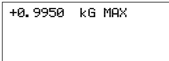
Assuming we are using a probe attached to the X axis, the maximum reading captured was 0.9950 kG, which is within the tolerance of the reference magnet. The reading will change as the probe moves around, but will eventually remain fixed on the highest reading. To recapture a new maximum value, press the **Max Reset** key.
