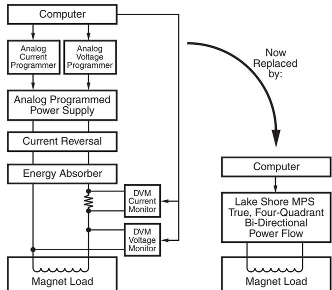
Figure 1-2. Comparison of Old and New MPS Designs
