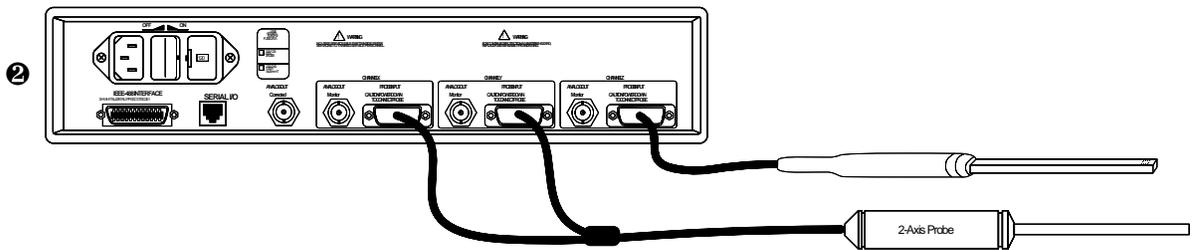
The Model 460 configured as 2 separate gaussmeters.
