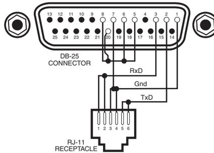
**Figure 5-5. Model 2002 RJ-11 to DB-25 Adapter Wiring**
