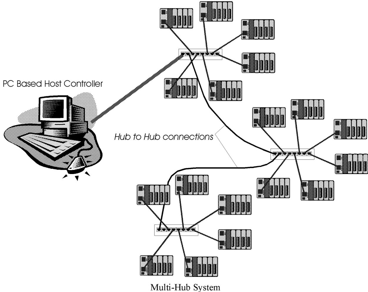
In a multi-hub system, all connections between the PC and a hub, or an RTU and a hub are straight-through. All connections between hubs are crossover.
