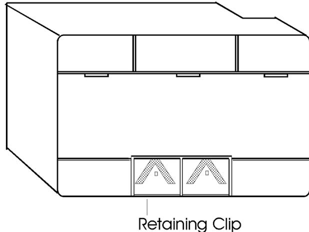
As shown in the figure, there is a DIN rail channel that runs lengthwise across the middle of the RTU base’s bottom side. At the top of that channel are three overhanging hooks. At the bottom of the channel there is a sliding retaining clip.
