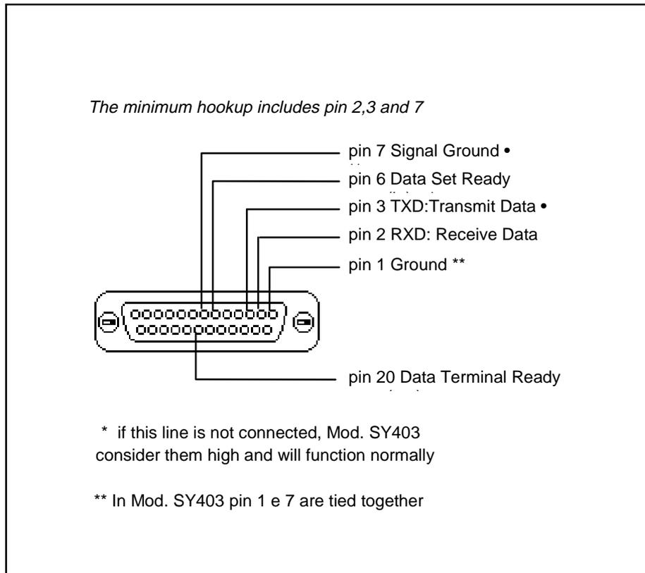
**Fig 3.2 RS232 connector pin assignment**
