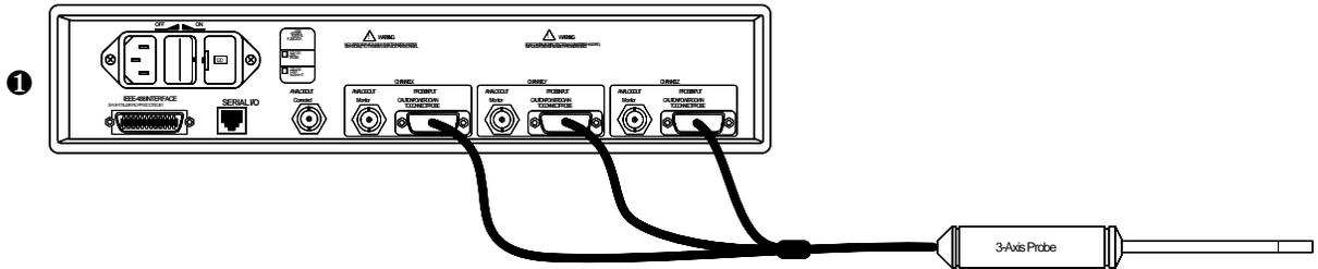
The Model 460 configured as a 3-axis gaussmeter.
