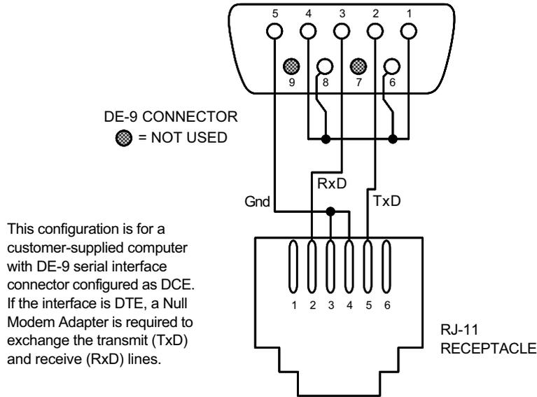
**Figure 6-8. Model 4003 RJ-11 to DE-9 Adapter Wiring Details**
