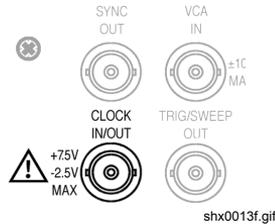
As an input it can be used either to run the instrument from an external master clock or as a synchronization input when slaved to another instrument as the master.
