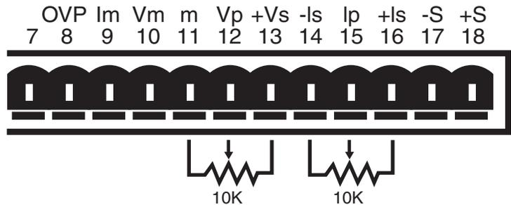
**Figure 2-2. Analog Monitoring , Programming, and Remote Sense Connections**
