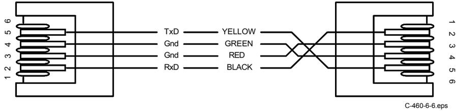
**Figure 6-6. Model 4001 RJ-11 Cable Assembly Wiring Details**
