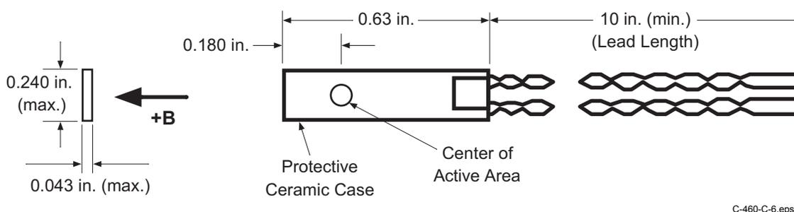
Figure C-6. Transverse Hall Generator HGT-3010, HGT-3030, and HGCT-3020 Dimensions
