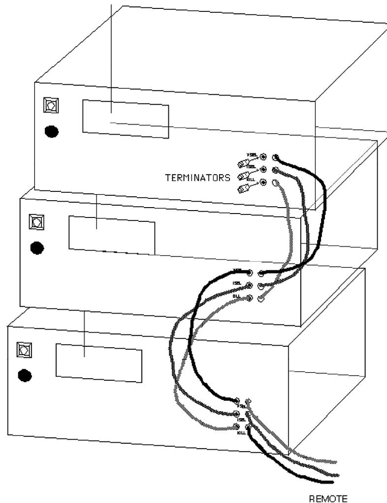
**Fig. 3.1 Connecting the Main controllers**
