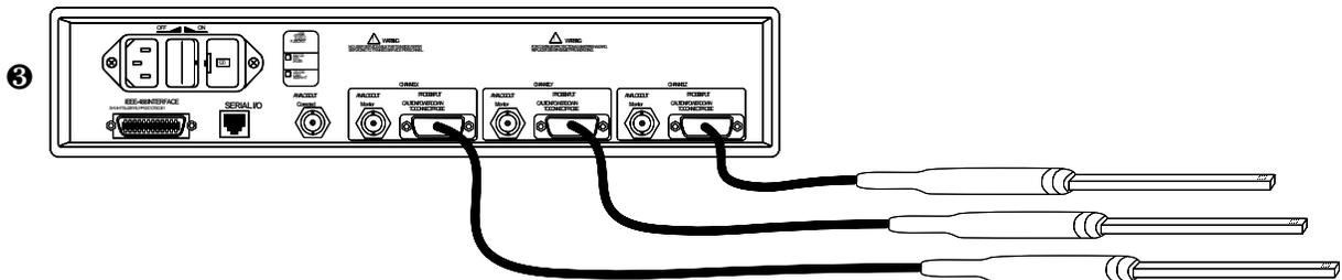
The Model 460 configured as 3 separate gaussmeters.
