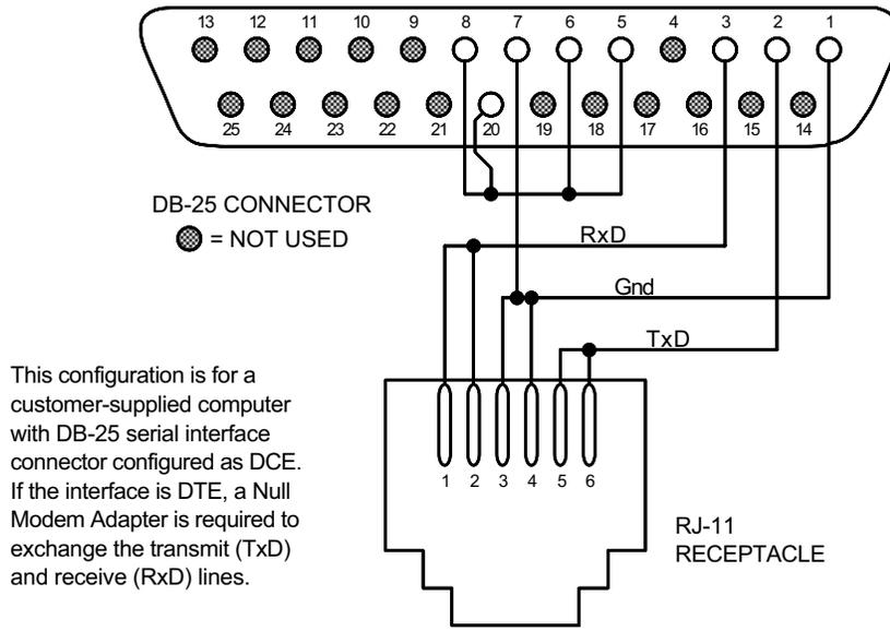
**Figure 6-7. Model 4002 RJ-11 to DB-25 Adapter Wiring Details**
