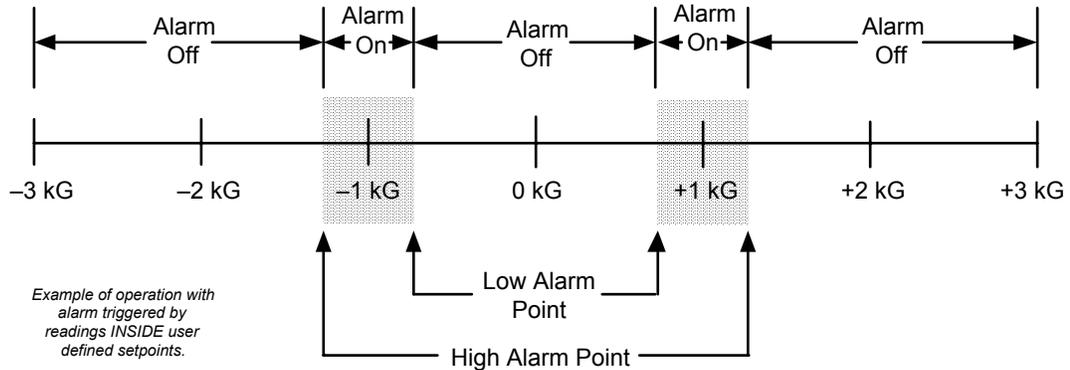
To enter this alarm setup, push the **Alarm Set** key. The user is asked to enter the High Alarm Point:
