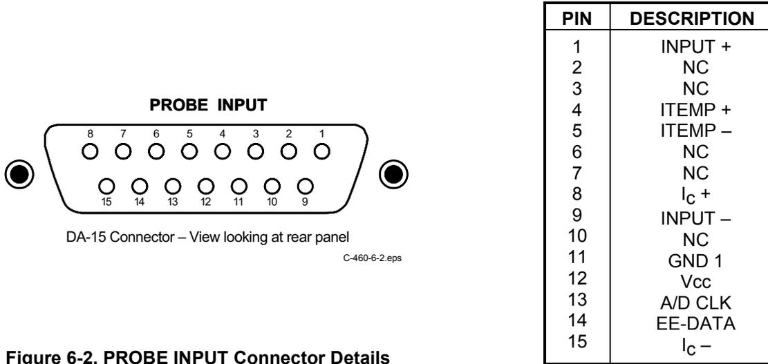
**Figure 6-2. PROBE INPUT Connector Details**
