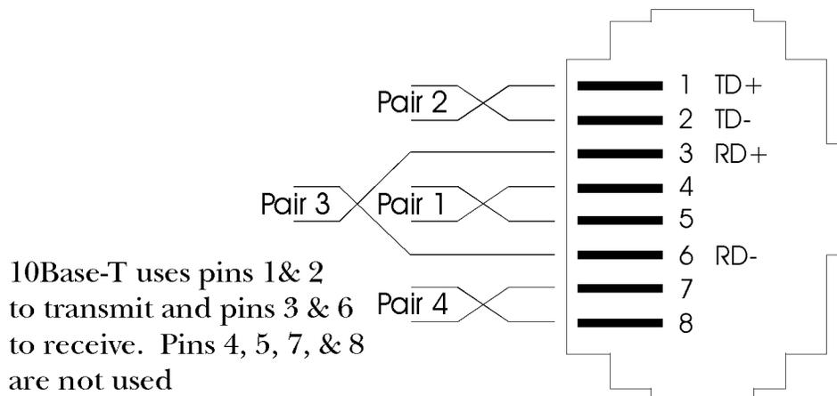
**Warning:** Do not attempt to save money by using two pair or flat type cable with RJ45 connectors. The RJ45 connectors will not securely fasten onto the cable jacket.
