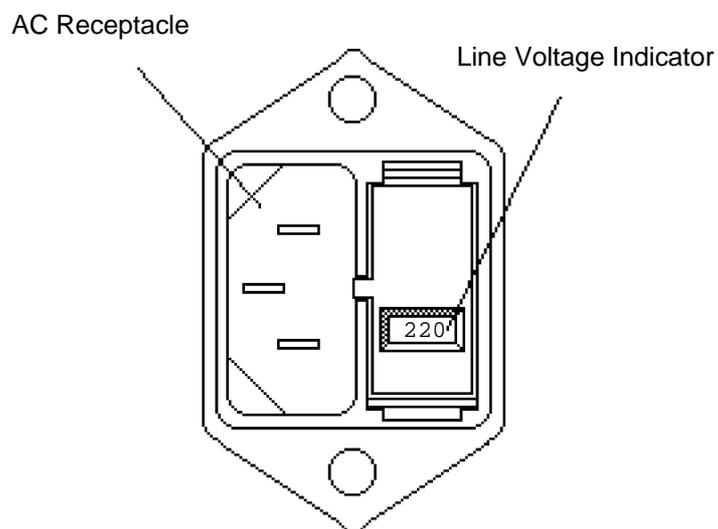
**Fig C.2: Operating Voltage Indicator**
