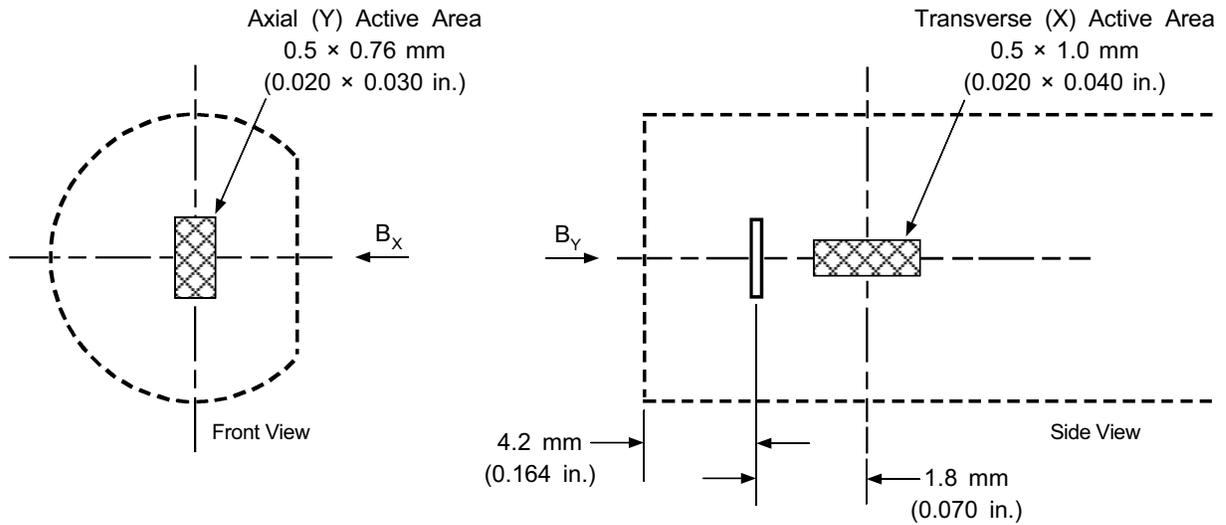
**NOTE:** Active area is defined as the portion of the Hall plate where the majority of magnetic sensitivity occurs. All position dimensions of the active area adhere to a tolerance of  $\pm 0.25$  mm (0.010 in.). Each active area is perpendicular to the other two to within  $\pm 0.5^\circ$ .
