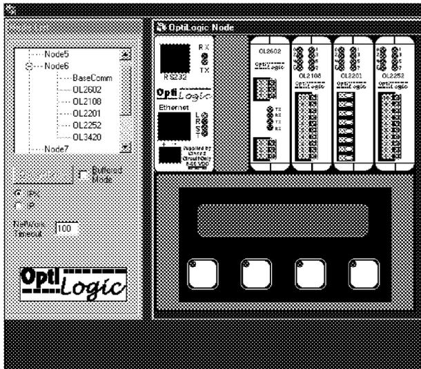
Click on a particular module, and its associated function screen will pop up. The figure below shows the function screen for the OL2108 relay output module, located in slot 0.
