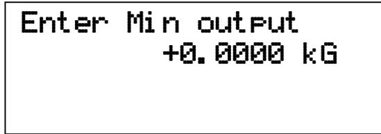
Enter the numbers 0.0 on the numerical keypad and press the **Enter** key. A minimum output of 0.0 kG has now been placed into memory. Changes to the Corrected Analog Output are immediately observable.
