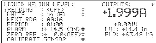
The cursor up and down keys move the line indicator. The ⬆ icon indicates parameters changed only with the Data Entry up and down arrows. When there are <ON> or <OFF> indicators, the Data
