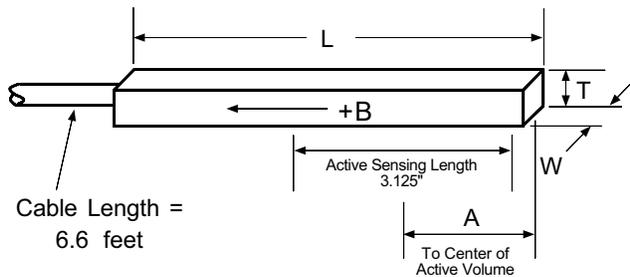
Small variations in, or low values of large volume magnetic fields, such as that of the Earth or fringe fields, around large solenoids, can be measured with these ultra-high sensitivity probes. Resolutions of several gammas ( $10^{-5}$  gauss) to tens of gammas are available depending on the mating gaussmeter.
