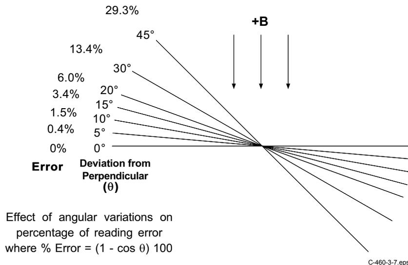
Figure 3-7. Effect Of Angle On Measurements
