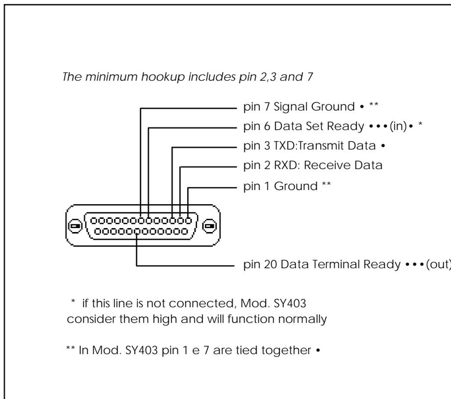
**Fig C.1 RS232 connector pin assignment**
