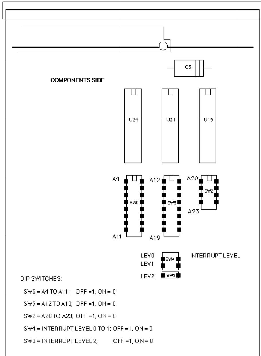
**Fig 6.1 V288 dip switches setting**
