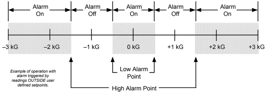
To enter this alarm setup, push the **Alarm Set** key. The user is first asked to enter the High Alarm Point as follows:
