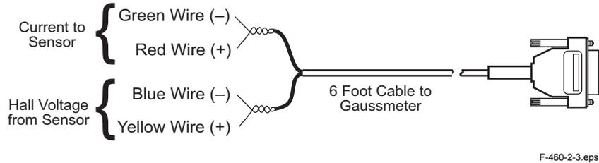
**Figure 2-3. Model MCBL-6 User Programmable Cable Accessory**
