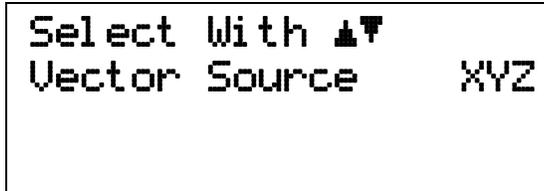
Use the **▲** or **▼** arrow keys to toggle the vector source between XYZ, XY, XZ, YZ, and X-Y. Press the **Enter** key to select a new setting, or press the **Escape** key (or wait for the timeout) to exit and retain the old setting. The vector source will be shown in the normal display. However, if Max Hold is selected for the vector magnitude display, the identifier MAX will appear in the normal display instead of the vector source.
