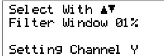
The filter limit window sets a boundary for restarting the filter. If a single field reading is different from the filter value by more than the limit specified, the instrument will assume the change is intentional and restart the filter at the new reading value. This allows the instrument to respond to changing fields much faster than if the filter functioned continually. Filter Window can be set from 1% to 10% of the present range.
