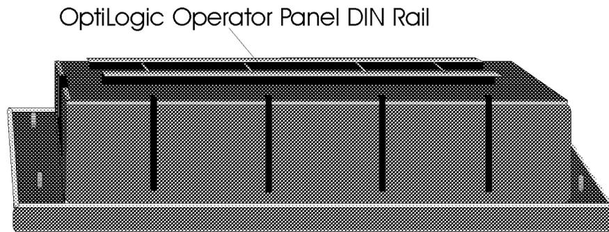
The mounting process is exactly the same as described for mounting to a DIN rail. Be sure that your orientation is right so the connectors on the base and the front panel line up. An OptiLogic RTU base attached to an OptiLogic operator panel should look like the figure below.
