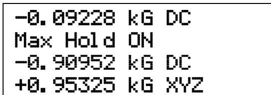
After a short timeout, the Y channel display will return to normal, with the Max hold value being displayed on the second line of the display as seen in the following display.
