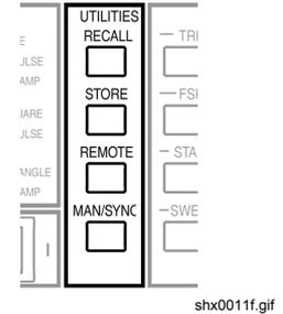
The **MAN/SYNC** key is used for manual triggering and synchronizing two or more generators when suitably connected together. Further information on synchronizing two generators is given in the *Users Manual*.
