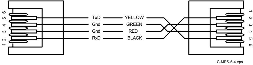
**Figure 5-4. Model 2001 RJ-11 Cable Assembly Wiring**
