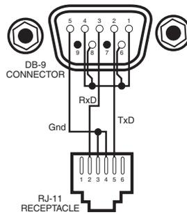
**Figure 5-6. Model 2003 RJ-11 to DB-9 Adapter Wiring**
