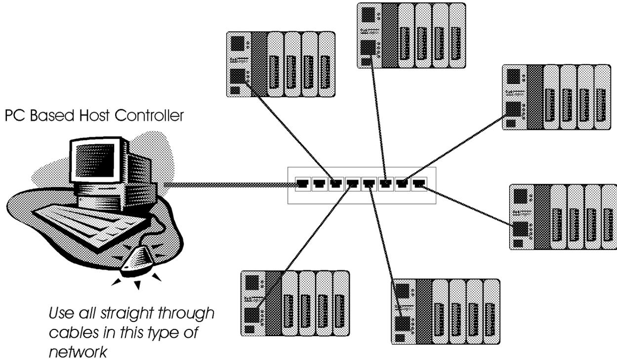
Crossovers are made internal to the hub. Therefore, in a single hub system, all connections are straight-through. Remember that for 10Base-T, each cable connection is limited to 100 meters in length.
