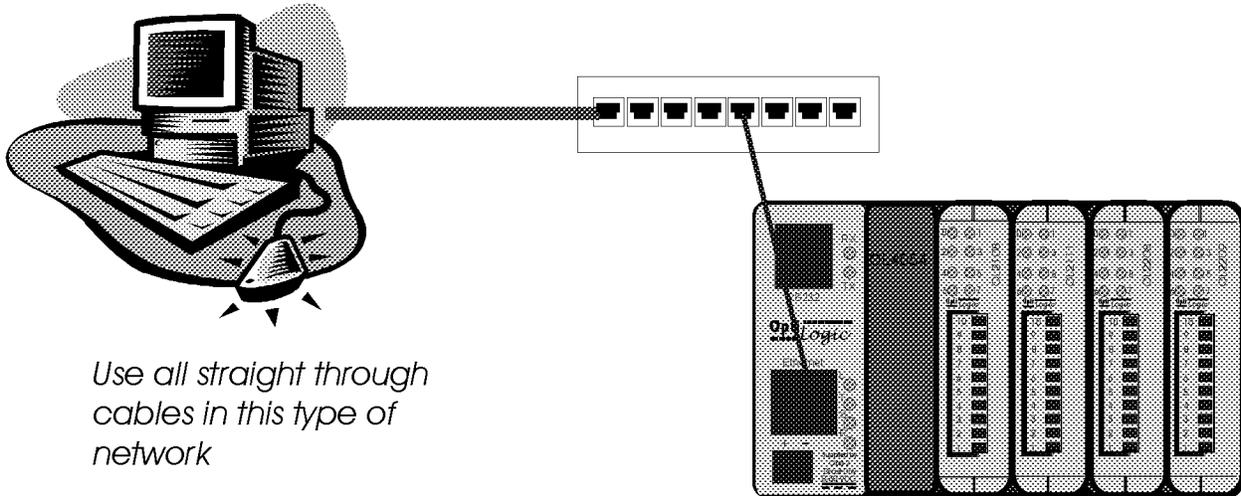
In either configuration, the first thing to check is if “Link” lights appear on the RTU. If you are connecting through a hub, link lights should appear on both the RTU connection and the PC connection. If the link lights do not appear you probably have a bad connection.
