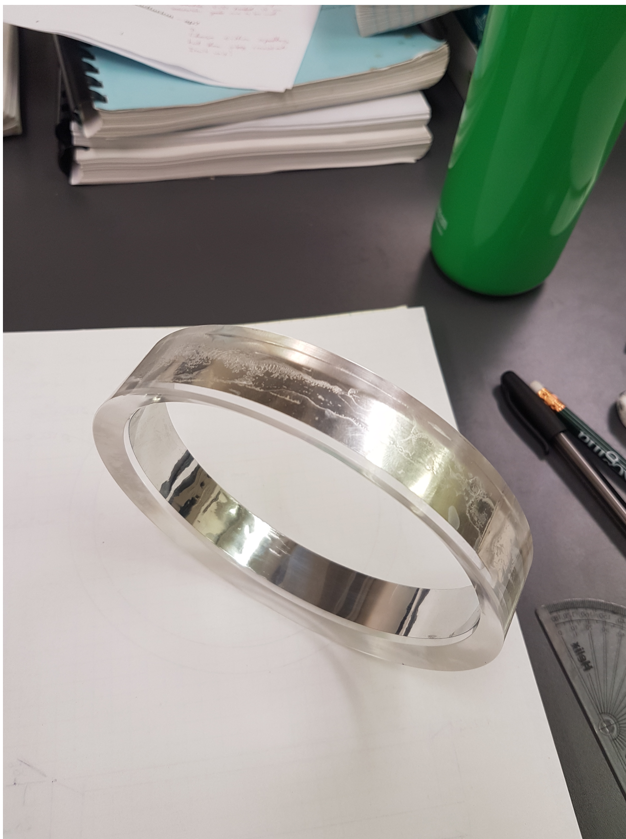
Figure 12: Side view of new optical object. Notice that the layer of aluminum is short of beveled surface to ensure no contact is made with PMT glass.
