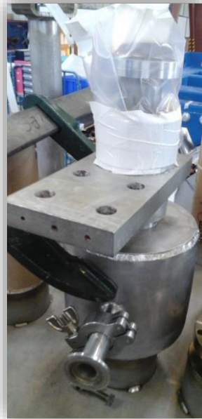
Figure 4: tooling for the leak test on VCL
