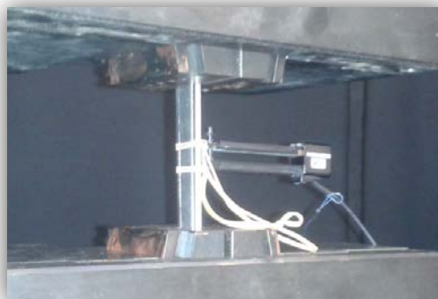
Figure 7: traction test on bare conductor consolidated at 2,95mm
