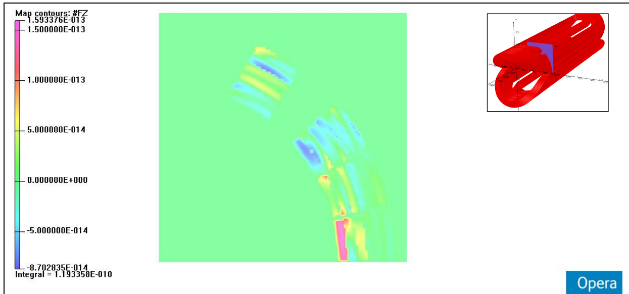
Fig. 19 –Fz force density in N/cm^3 - Integrated Fz force in N/m – 3419.4 A
