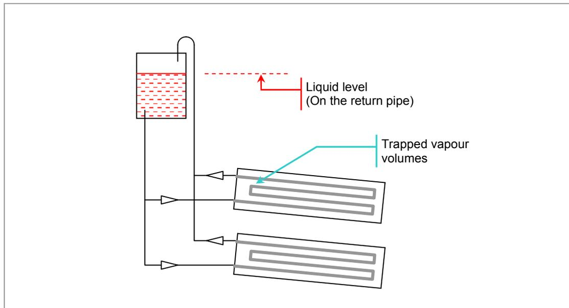
The return pipe opens above the liquid level in the reservoir. There will be a matching liquid level in the return pipe. Therefore the return will be vapour: the vapour bubbles will be generated on the radiation screen and then rise through the liquid to return to the reservoir. However high points on the screen will create trapped volumes of vapour.
