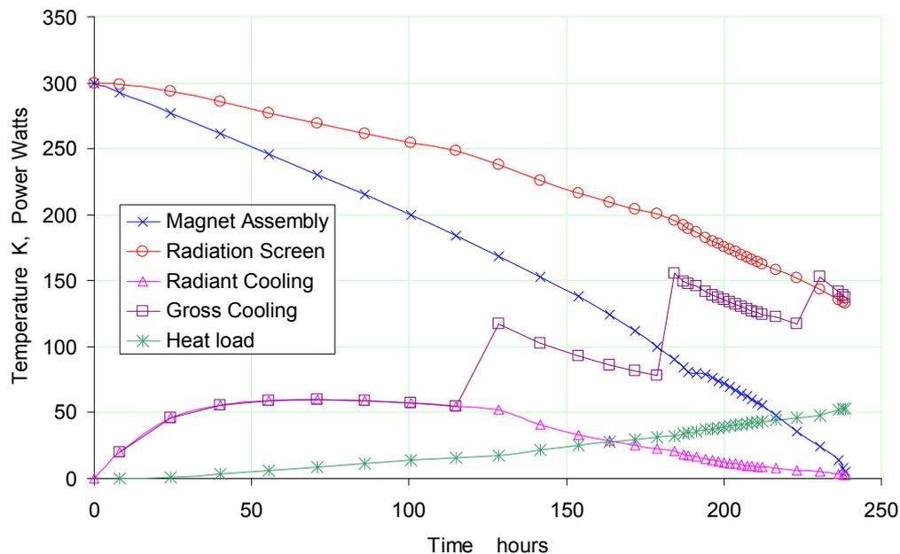
The purple line (squares) show the nitrogen cooling power increasing (in discrete increments) and cooling the screen to below 130 K at which point the danger of thermal shocks is minimised.
