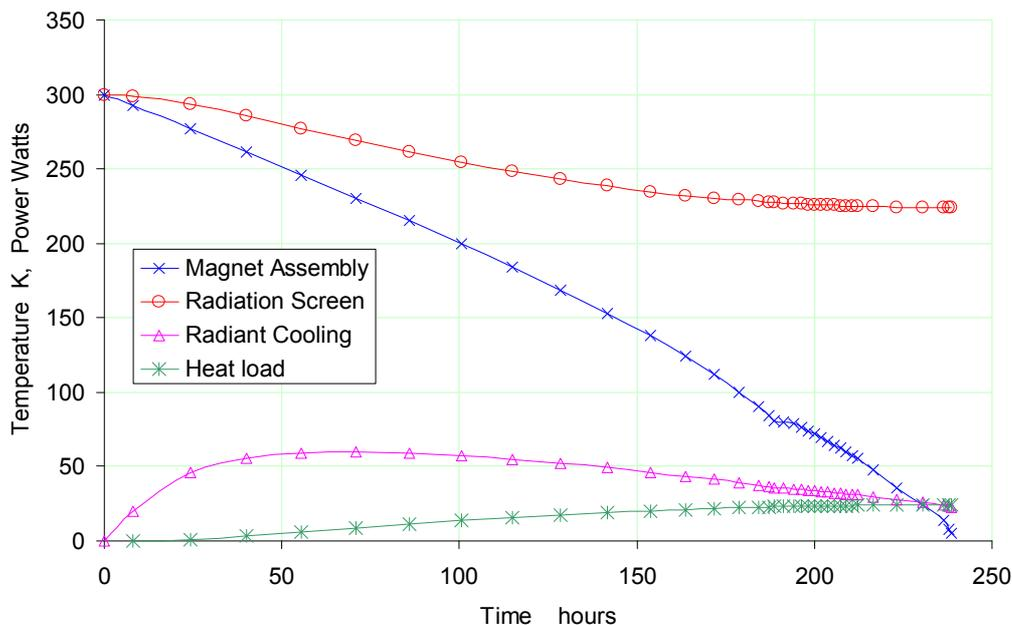
The radiation screen will equilibrate at about 220 K which is still too warm to continue the cooling with liquid nitrogen without a danger that thermal stresses will cause distortion and damage to the screen.
