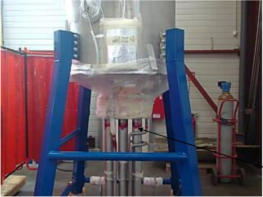
PT on 10 welds
