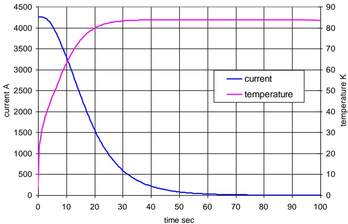
Fig 4: unprotected quench, ignoring the spacer between coils A and B
