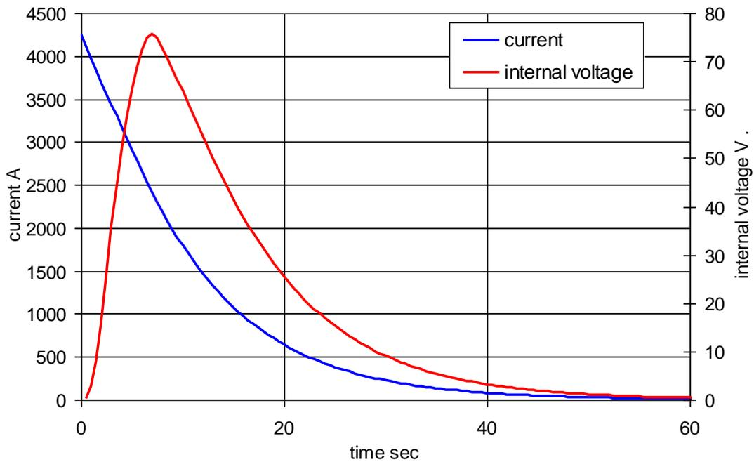
Fig 7: current and internal voltage for quench of Fig 6.
