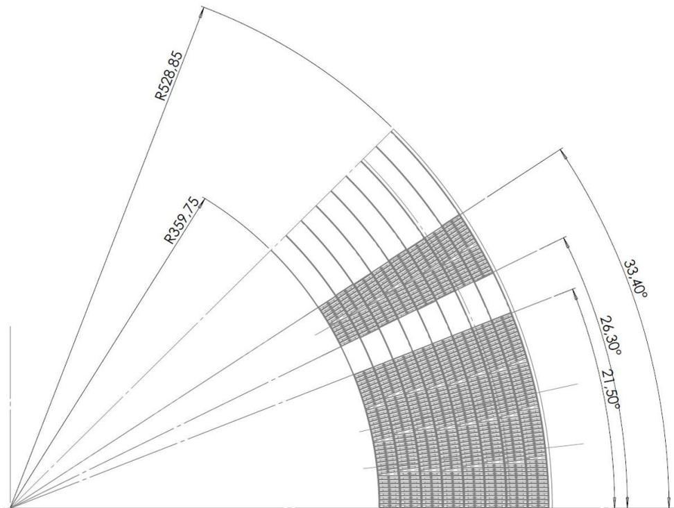
inner radius  $r_i := 359.75 \text{ mm}$     outer radius  $r_o := 528.85 \text{ mm}$     radial thickness  $t_{rA} := r_o - r_i = 16.91 \text{ cm}$
