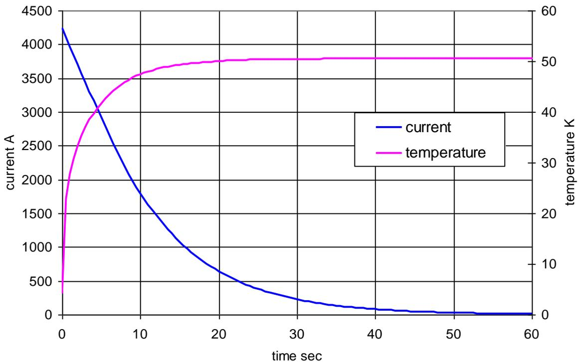
Fig 6: protected quench, ignoring the spacer between coils A and B
