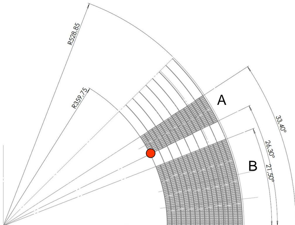
Fig 1: Cross section of the coils: quench assumed to start at red dot
