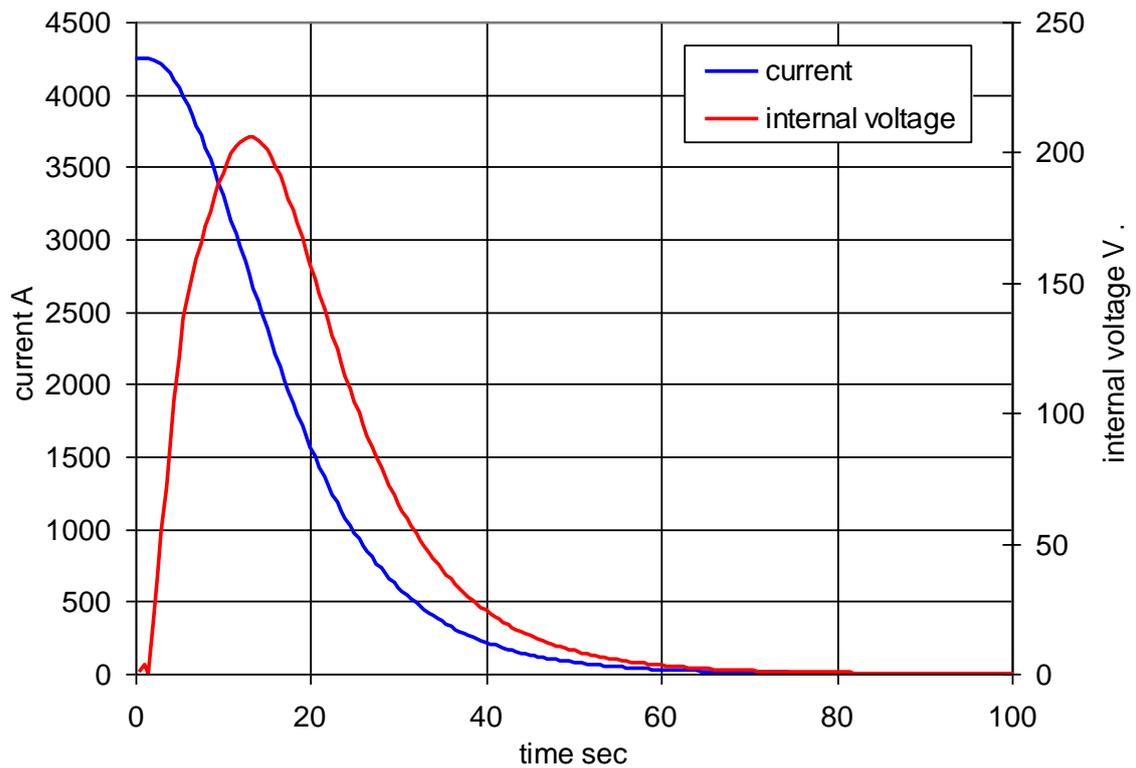
Fig 5: current and internal voltage for quench of Fig 4.
