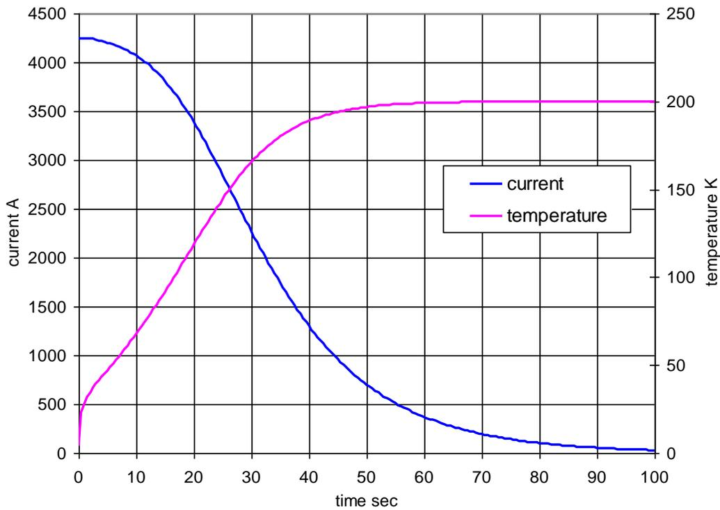
Fig 2: unprotected quench with resistive zone confined to coil A
