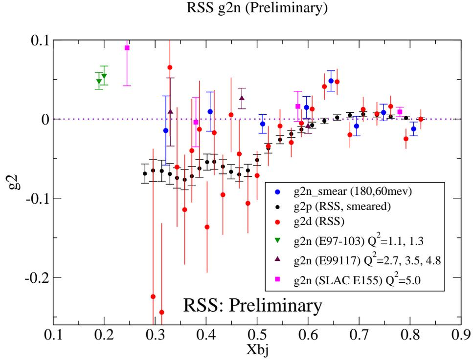
Figure 8: Preliminary results of  $g_2^n$  extracted from RSS deuteron  $g_2$  (data) and smeared proton  $g_2$ . Our results basically agree with the world data measured at the DIS regime, and are also consistent with zero except for one data point at  $x_{BJ} = 0.65$ .
