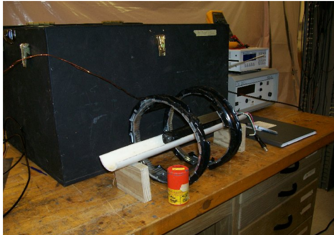
Figure 13: The PMT is shown resting in its trough within the helmholz coil. Behind sits the blackbox within which the testing takes place. The electronics rack is not shown here.
