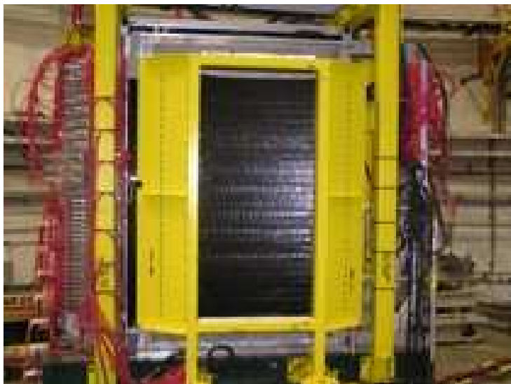
Figure 5: Front view of the Lucite Hodoscope. The last bar is missing.
