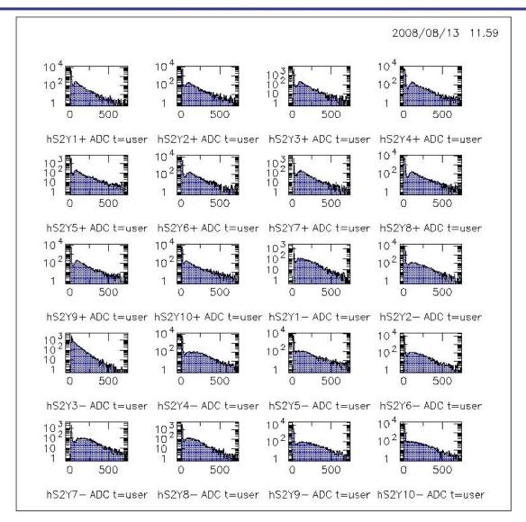
ADC signals from HMS hodoscope 2Y plane
