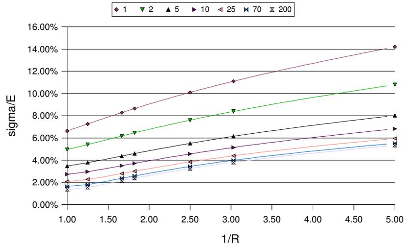
Figure 1. Energy resolution as a function of glass transparency for energies from 1 to 200 GeV.
