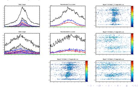
Red is Y1, blue is Y2, black is both, and Delta = (raster-recon) Now with X plane in *front*, and tracker positioned at 52cm Adding a correction to Y1 and Y2 positions by moving them closer together by 14 mm
