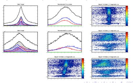
Red is Y1, blue is Y2, black is both, and Delta = (raster-recon) Problem: The target reconstruction in the X-Z plane at the target is different between Y1 and Y2. Adding a correction to Y1 and Y2 positions by moving them closer together by 8 mm
