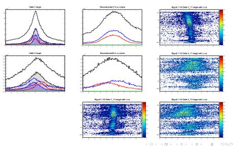
Red is Y1, blue is Y2, black is both, and Delta = (raster-recon) Problem: The target reconstruction in the X-Z plane at the target is different between Y1 and Y2. Moving back the whole detector to 52cm
