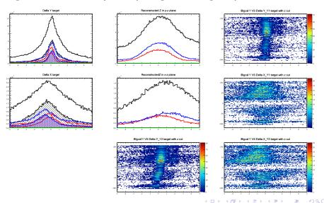
Red is Y1, blue is Y2, black is both, and Delta = (raster-recon) Problem: The target reconstruction in the X-Z plane at the target is different between Y1 and Y2. Adding a correction to Y1 and Y2 positions by moving them closer together by 14 mm
