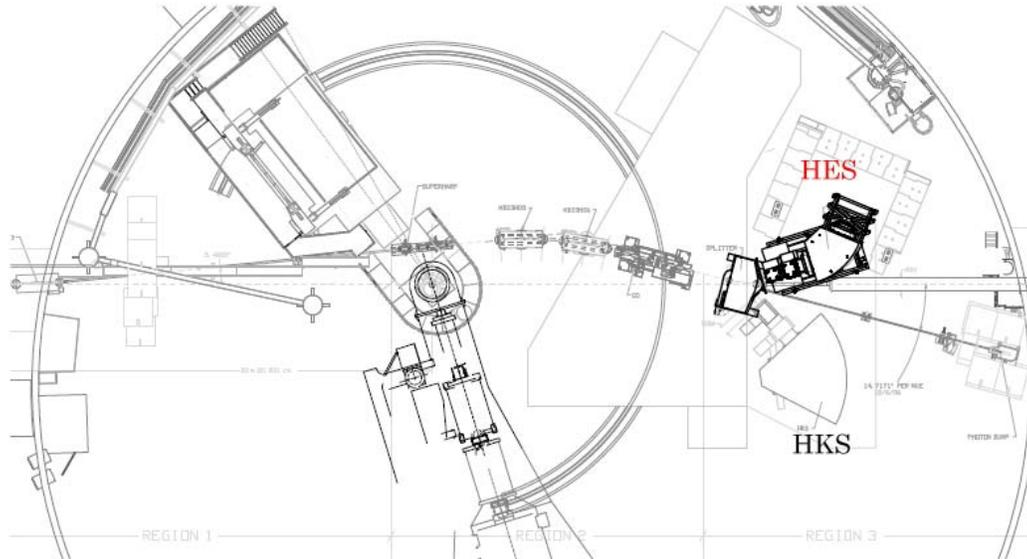
Figure 7: Floor plan of the HKS + HES + new SPL configuration in Hall C for the proposed experiment.
