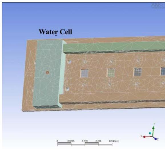
Figure 10: Schematic figure of a target ladder with a water cell. Pockets can accept  $1 \times 1\text{cm}^2$  solid targets and one of them is replaced by a water cell which is connected to cooling water pipes.
