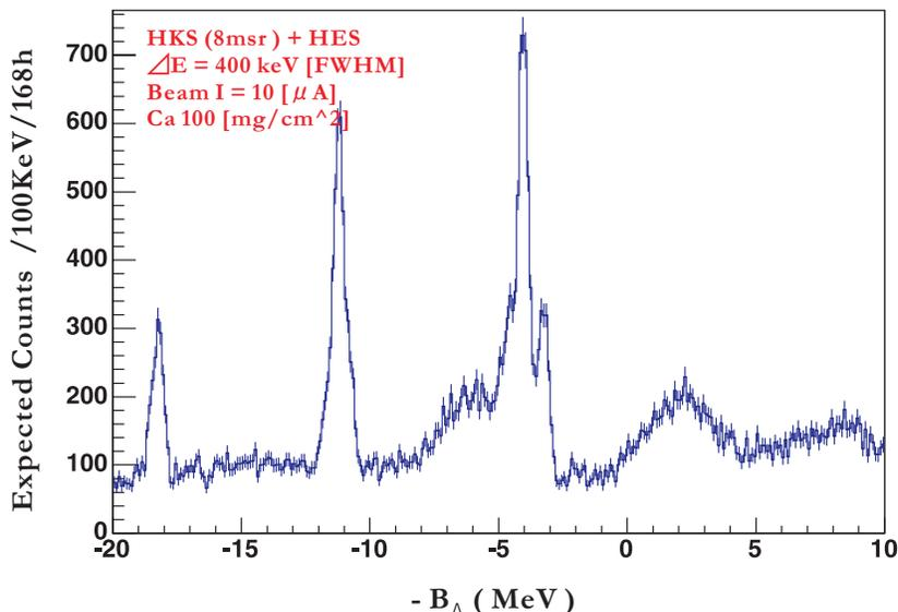
Figure 9: An expected  $^{40}\text{Ca}(e,e'\text{K}^+)_{\Lambda}^{40}\text{K}$  spectrum. The HKS-HES acceptance was taken into account in the GEANT simulation. Quasi-free events expected in  $-B_{\Lambda} > 0$  are not included.
