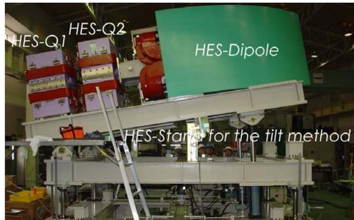
Figure 6: Completed HES magnets in Sendai, Japan. HES EQ1-EQ2-ED magnets are placed on the tilting support frame.
