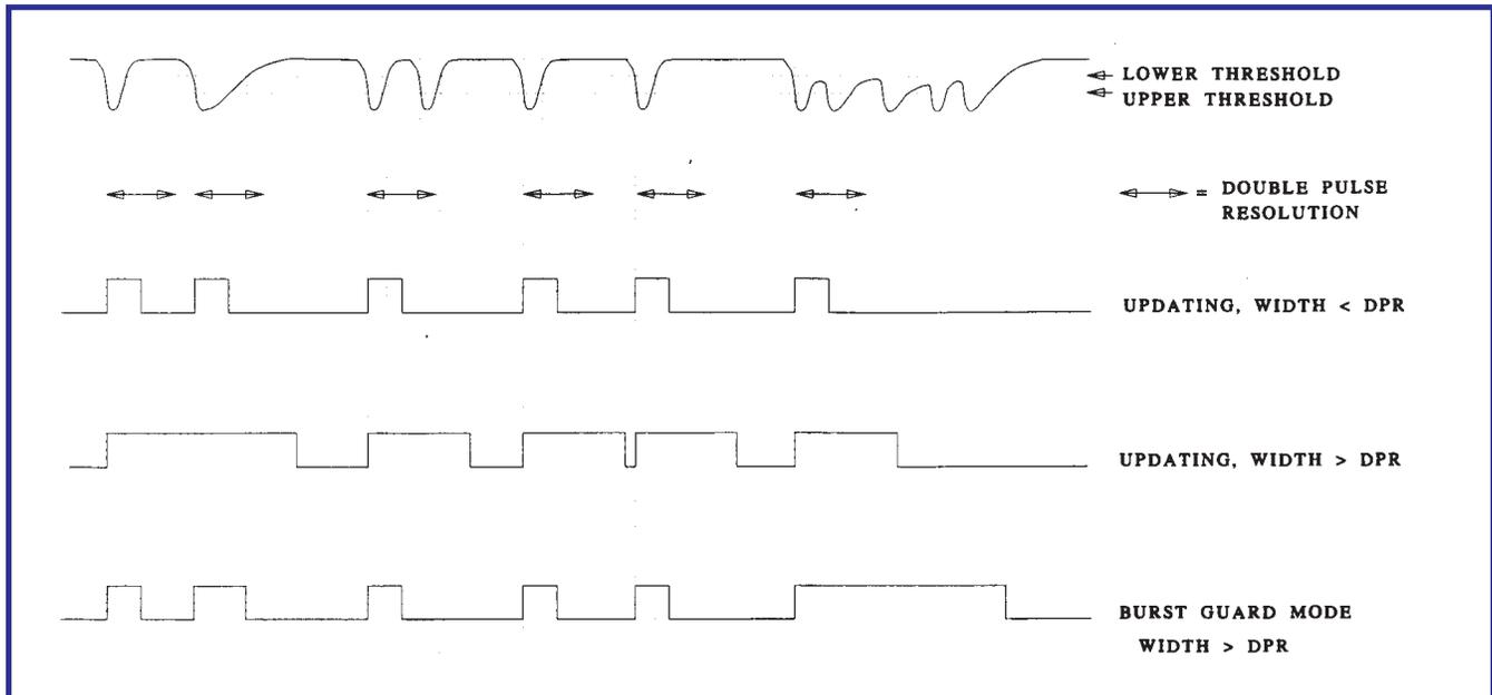
Model 4413 Output Modes. Comparison of Updating and Burst Guard Modes with various fast input signals. DPR is the Double Pulse Resolution Interval set to minimum in this example.
