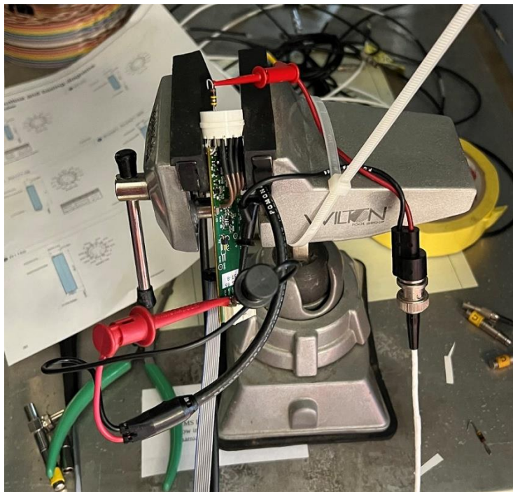
Figure 4 Bench view of how the pulser signal is injected into the PMT anode through a large resistance. (Near the top.) The resistor lead is cut to about half length, folded into a V shape, and plugged more or less securely into the PMT socket.
