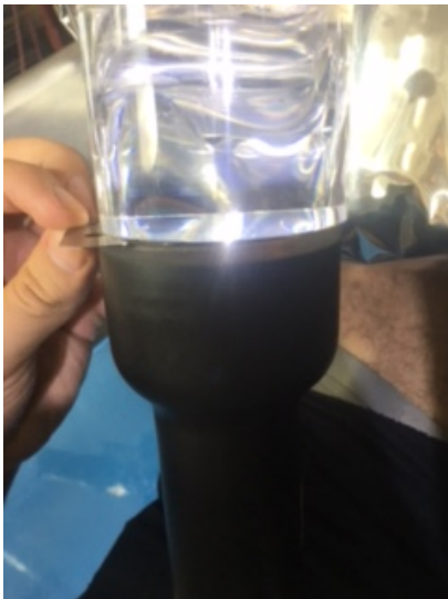
Figure 13 Blade placement for removing PMT
